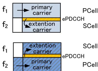
**Figure 8: LTE-A HetNet using CA and an Enhanced PDCCH Control Channel**
