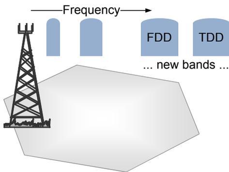
**Figure 10: Increase of Available Bands and Band Combinations for Carrier Aggregation**
