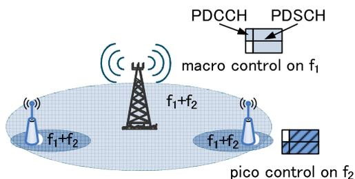
**Figure 5: LTE-A HetNet using CA in a Co-channel Deployment Scenario**
