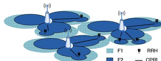
**Figure 2: LTE-A HetNet using Co-Channel Deployment**
