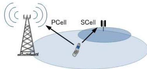
**Figure 4: LTE-A HetNet Multi-site Carrier Aggregation**
