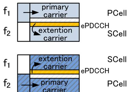
**Figure 9: LTE-A HetNet using CA and ePDCCH with Interference Coordination**
