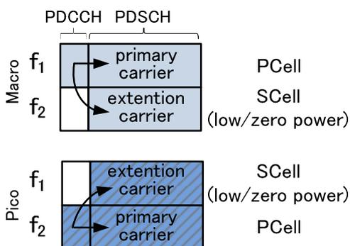
**Figure 6: LTE-A HetNet using CA with Cross Carrier Scheduling for PDCCH Protection**
