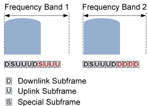
**Figure 11: TDD Carrier Aggregation with Different Subframe Configuration**
