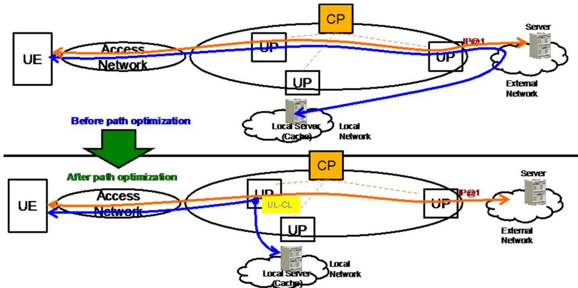
Figure 8: Depiction of offloading data to local cache using the concept of dedicated bearers [18].
