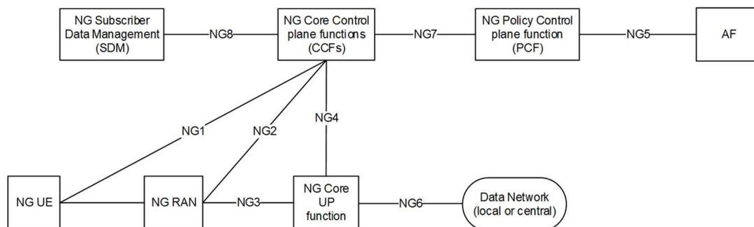
Figure 5: Overall architecture option as proposed by mobile vendors [7].
