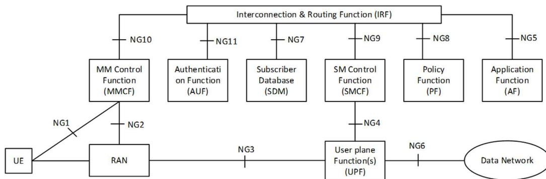
Figure 4: Overall architecture option as proposed by network operators [6].
