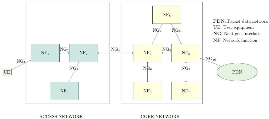
**Figure 2: Top-down approach of identifying network functions and the next-gen interfaces. Only an overall high-level architecture is proposed in this method. Network functions (NF) will be the building blocks of the future networks.**
