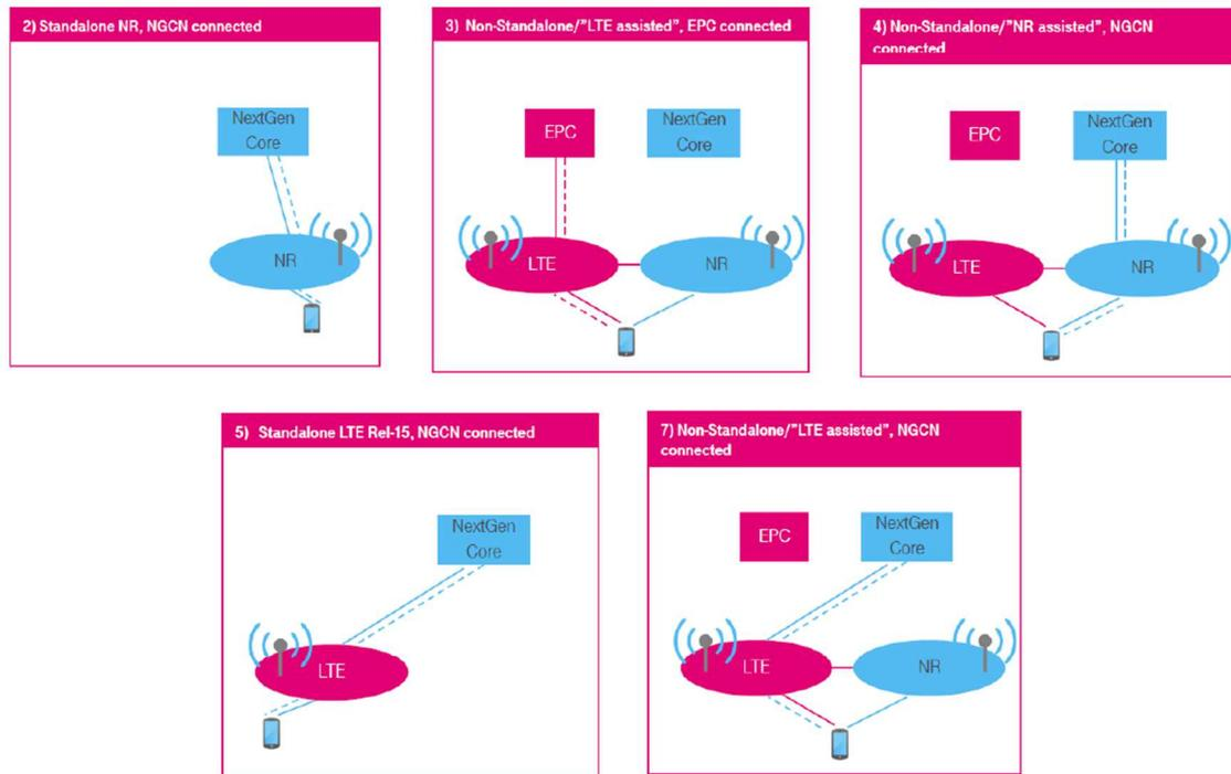
**Figure 9: Deployment perspective for future 5G networks [20].**
